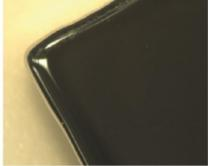
Layer thickness: ca. 4 µm Edge: ca. 6 µm Almost no pores.
