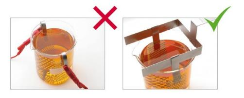
Features of Umicore beakerglass anodes are: easy handling, replaceable anode-segments.
