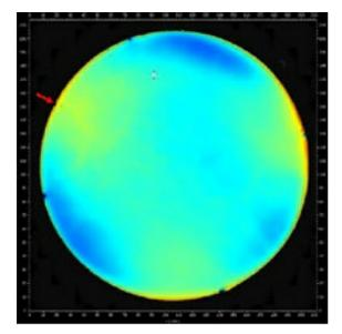
Very low stress of IntraCu® SC layers: 8 inch blanket wafer, plated on one side with 20 μm, shows warpage < 10 μm.
