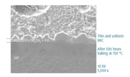
BGA Solder Ball Shear Results (ball size 0.76 mm, SAC solder, 4.8  $\mu$ m NiP, 0.15  $\mu$ m Pd, 0.06  $\mu$ m Au)
