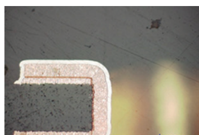
Cross section photo after OSP treatment
