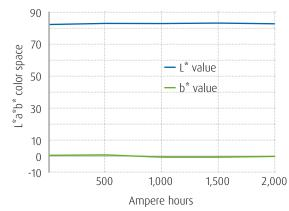
The coating results are not influenced by the anodes in terms of color. L\* value (brightness) and b\* value (color intensity between blue and yellow) are always at a constant level. The other coating properties are also not changed - even at maximum utilization.
