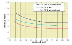
Typical dispersions of the refractive index of LATI<sup>™</sup> films for the indicated deposition conditions. IAD parameters for coatings on plastic substrates.
