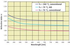
Typical dispersions of the refractive index of Zr-Ti-oxide films for the indicated deposition conditions. IAD parameters for coatings on plastic substrates.
