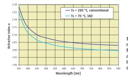
Typical dispersions of the refractive index of ROMA<sup>™</sup> films for the indicated deposition conditions. IAD parameters for coatings on plastic substrates.
