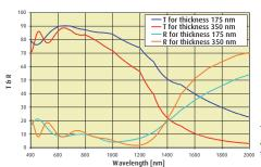
Typical transmittance and reflectance spectra for ITO.
