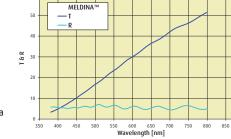
Typical transmittance and reflectance spectra for MELDINA<sup>™</sup>.
