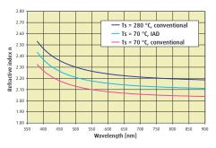
Typical dispersions of the refractive index of DRALO<sup>™</sup> films for the indicated deposition conditions. IAD parameters for coatings on plastic substrates.
