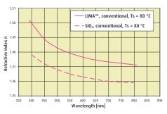
Typical dispersions of the refractive index of LIMA<sup>™</sup> films for the indicated deposition conditions.
